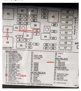
Install Coolit Relay in #43 slot. Install Coolit Fuse adaptor in fuse slot #15 like in picture below. (Relay in photo is a V3, V2 notch faces toward battery.
