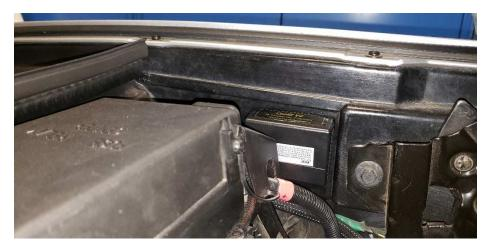
Connect long ground wire to ground stud on front of frame below Coolant reservoir like in photo below.
